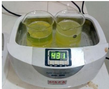
Fig 7. Mixture of CeO 2 & Bio Diesel Blends in Water Bath of Ultrasonicator
